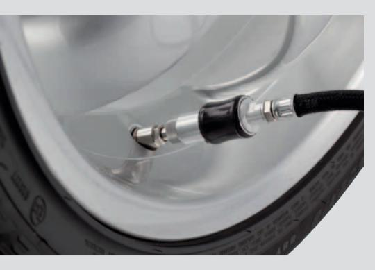
It is difficult to inflate a tyre with compressed air without routine and practice. Air can escape from the tyre very quickly if the standard valve coupling on the compressed air device (e.g. lever connector or clamp connector with tongue) is not seated precisely and sealed against the tyre valve.
