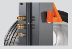
Variable compressed air connection at column side (figure) or top. Two distributors for connecting a tyre inflator or impact screwdriver.
