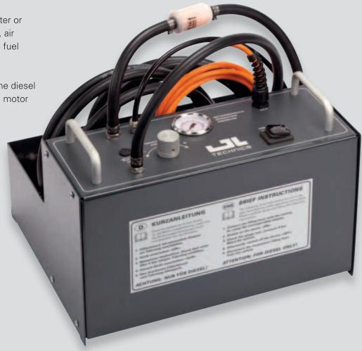
The electrical DEG diesel venting device enables rapid and safe venting of HDEP/MDEG diesel motors. It uses a high-performance pump to transport diesel fuel into the lines so that retained air is able to completely escape the fuel circuit.
